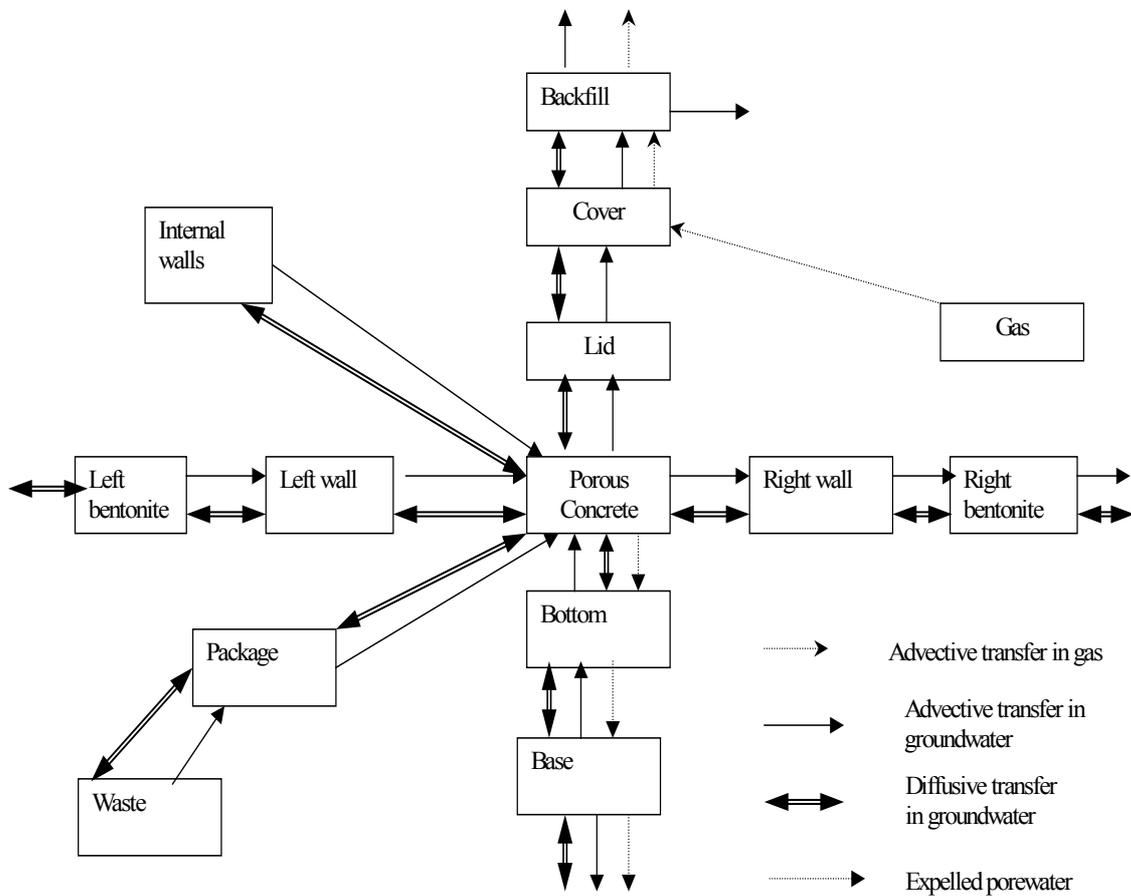
**Figure 6.6** The Silo Engineering Sub-Model
