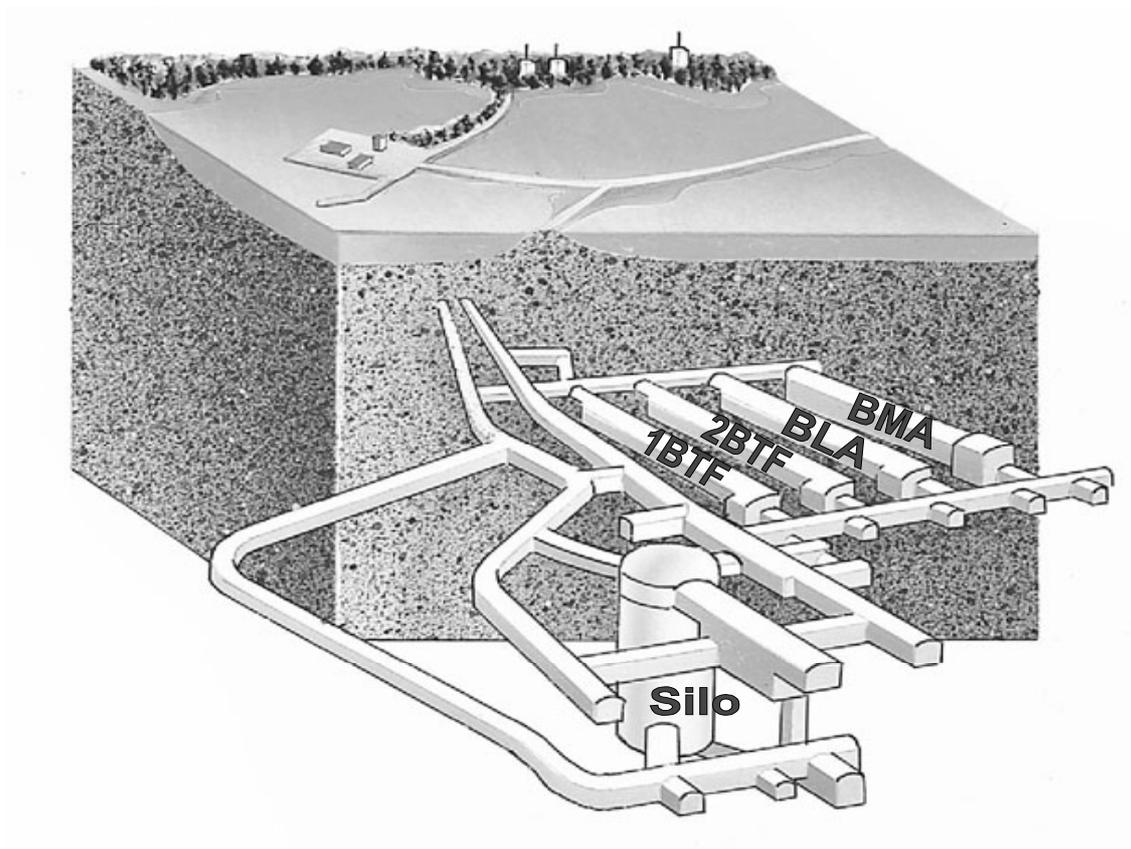
*Figure 2.1* Schematic illustration of the SFR 1 repository, showing the various vaults and the Silo
