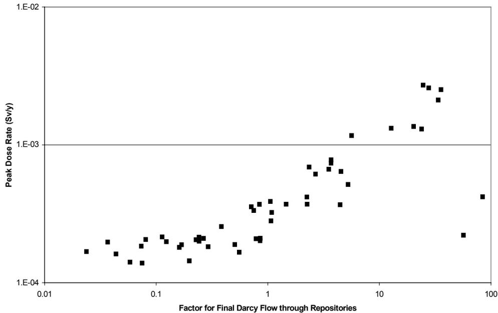
**Figure 6.13** Scatter Plot for Peak Dose Rate for Terrestrial Pathways against uncertainty factor for the Final Darcy Flow through the Vaults
