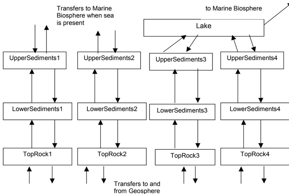
**Figure 6.8** *The Terrestrial Biosphere Sub-System*
