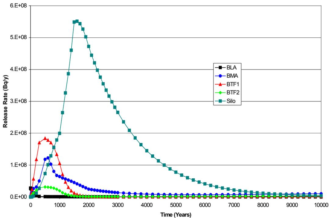
**Figure 6.10** Radionuclide Fluxes from the Vaults in the Reference Calculations
