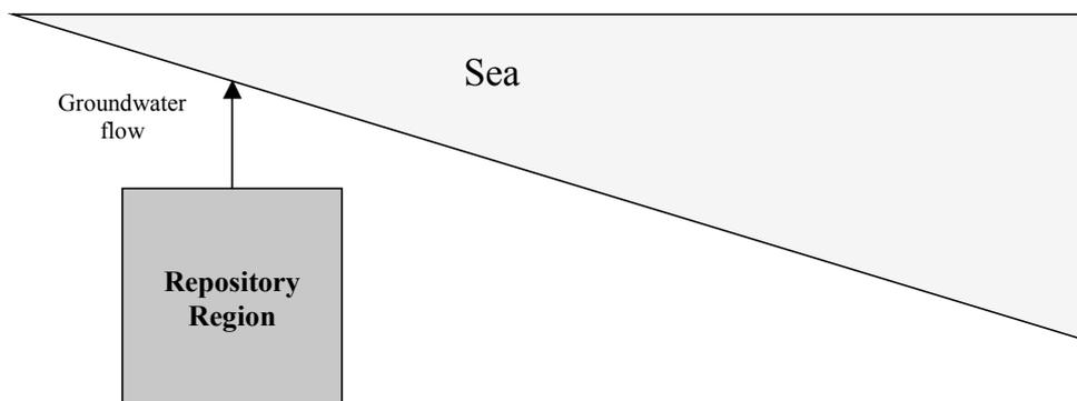
**Figure 6.3** *Groundwater Flows when the Repository is below the Baltic*
