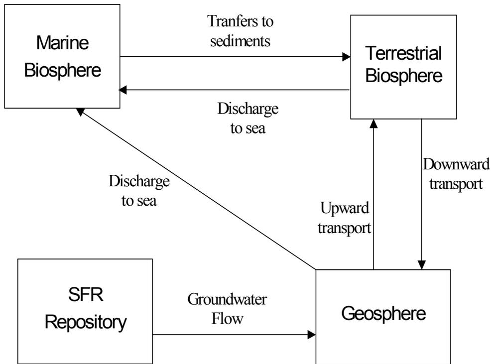
**Figure 6.1** *The AMBER System Model for SFR 1*
