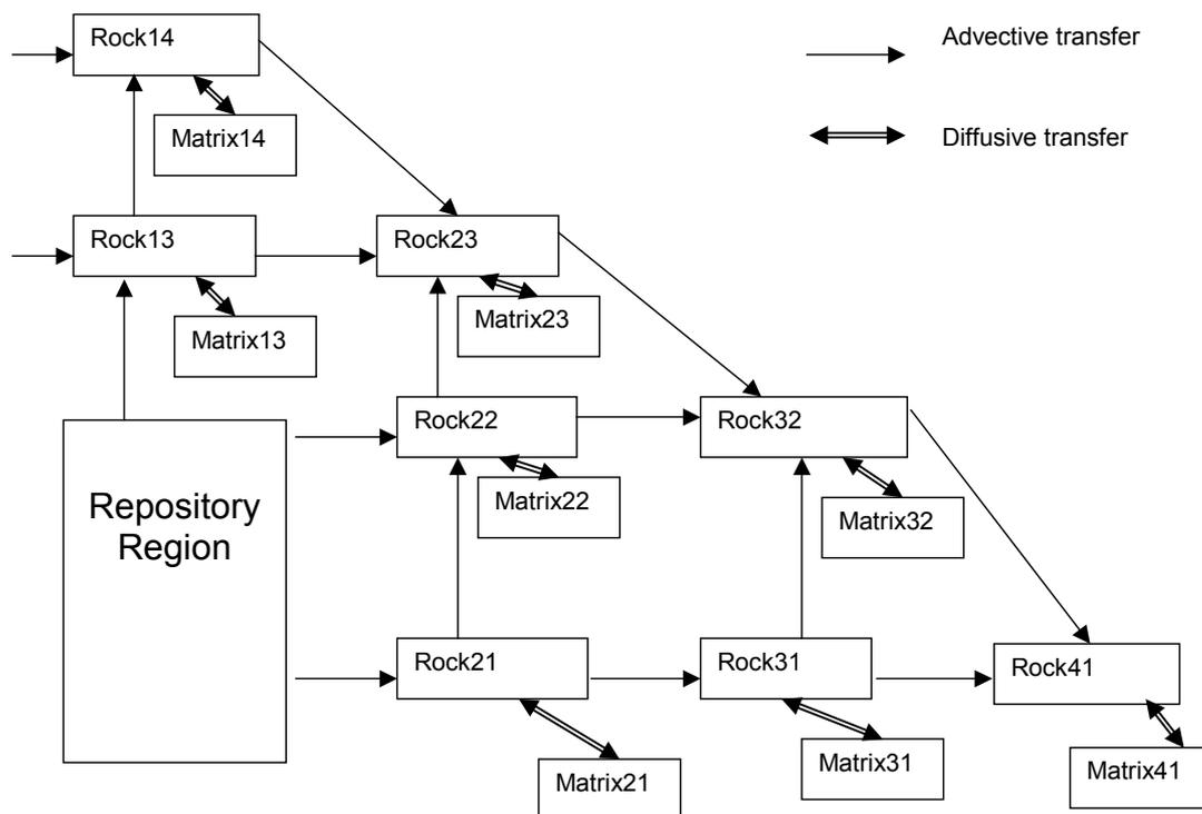
**Figure 6.7** *The Geosphere Sub-System*
