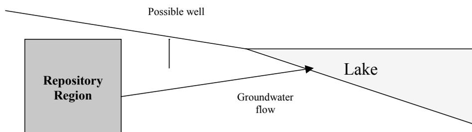
**Figure 6.4** *Groundwater Flows when the Baltic has Retreated*
