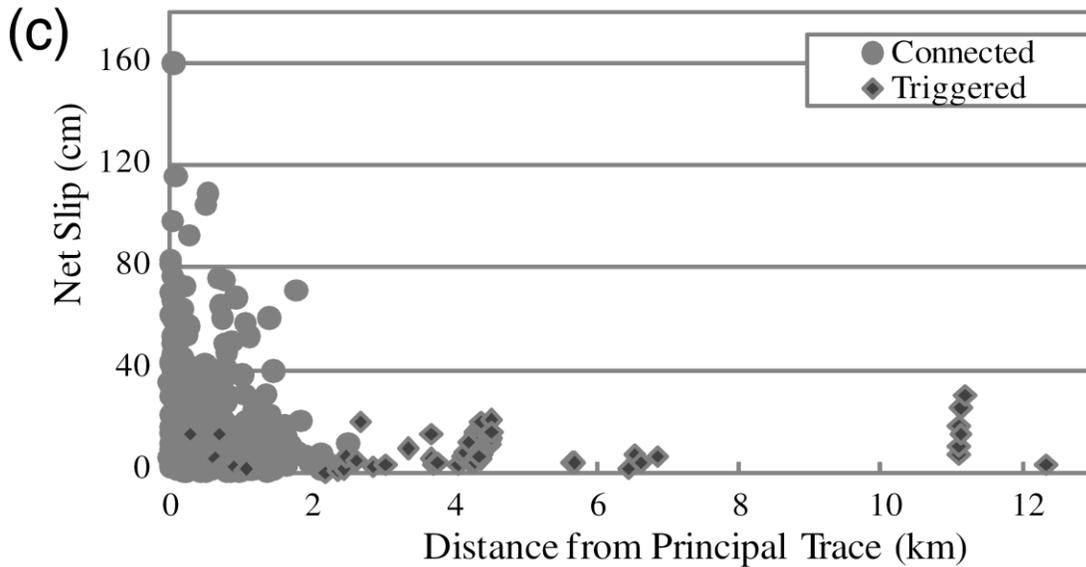
Fig. 13. Net slip on distributed faults during strike-slip surface ruptures, as a function of distance from the primary fault. Triggered faulting dominates beyond about 2 km from the primary fault. From Petersen et al., 2011, Fig. 2.
