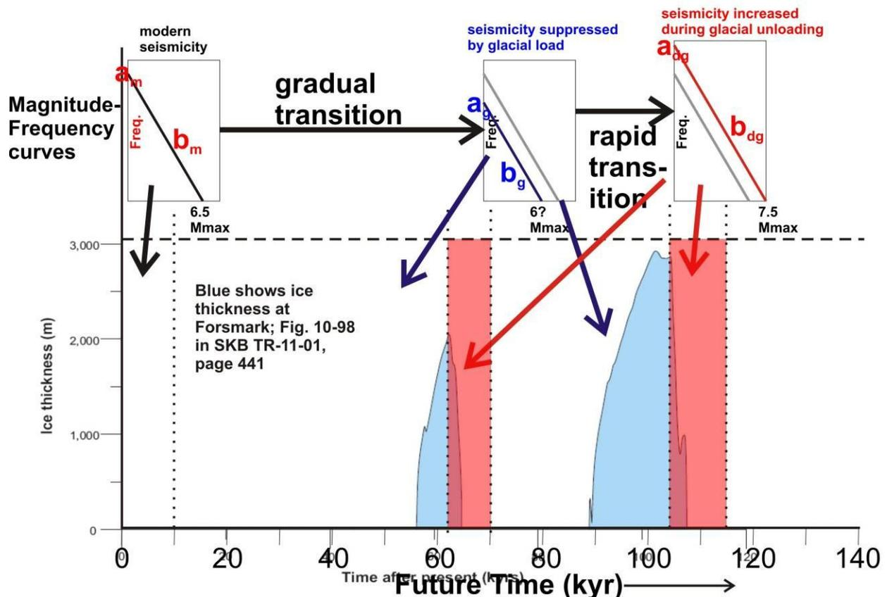
Fig. 6. Conceptual view of seismicity through the next 100,000-year glacial cycle. The lower half of the diagram shows the thickness of glacial ice at the Forsmark site (in blue) during the growth of the next ice cap. The red box marks the 10 kyr period of rapid deglaciation at the Forsmark site, when crustal rebound
