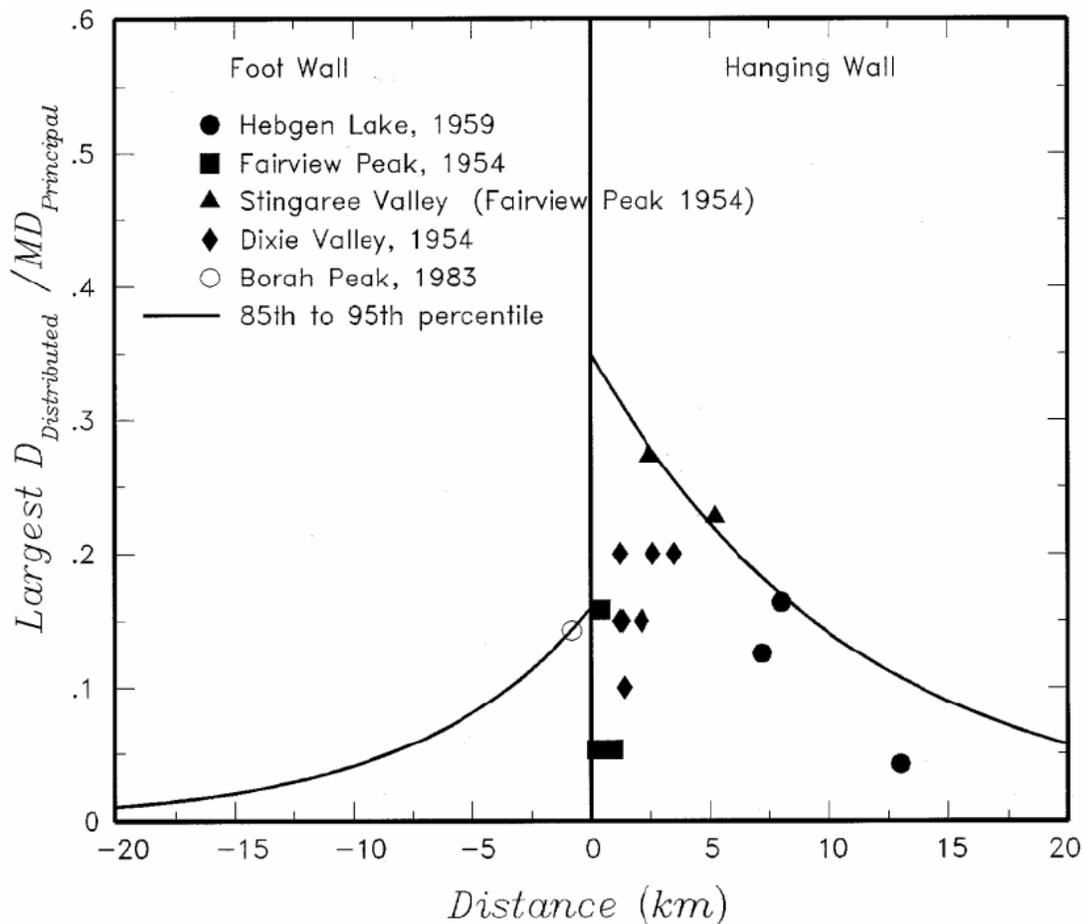
Fig. 12. Data for larger displacements on distributed ruptures divided by the maximum displacement on the principal rupture, for a set of five normal fault surface-ruptures in the USA. The curves represent a high percentile (e.g., 85th to 95th) of the distribution for  $D_{Distributed} / MD_{Principal}$ . The data were compiled by C. dePolo for the Yucca Mountain PSHA (Stepp et al., 2001).
