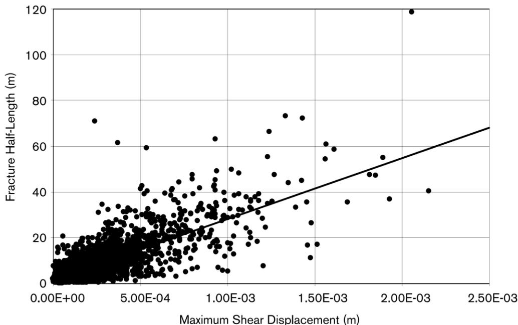
Fig. 15. Induced shear displacements in population of target fractures within box-shaped rock volume at 2 km distance from a fault generating a M6.1 strike-slip earthquake /from La Pointe et al. 1997/.
