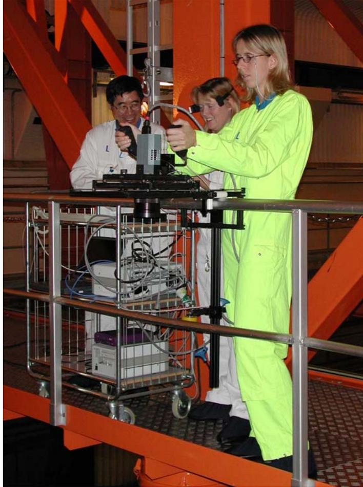
*Figure 3: Railing Bracket Mounted on Bridge*
