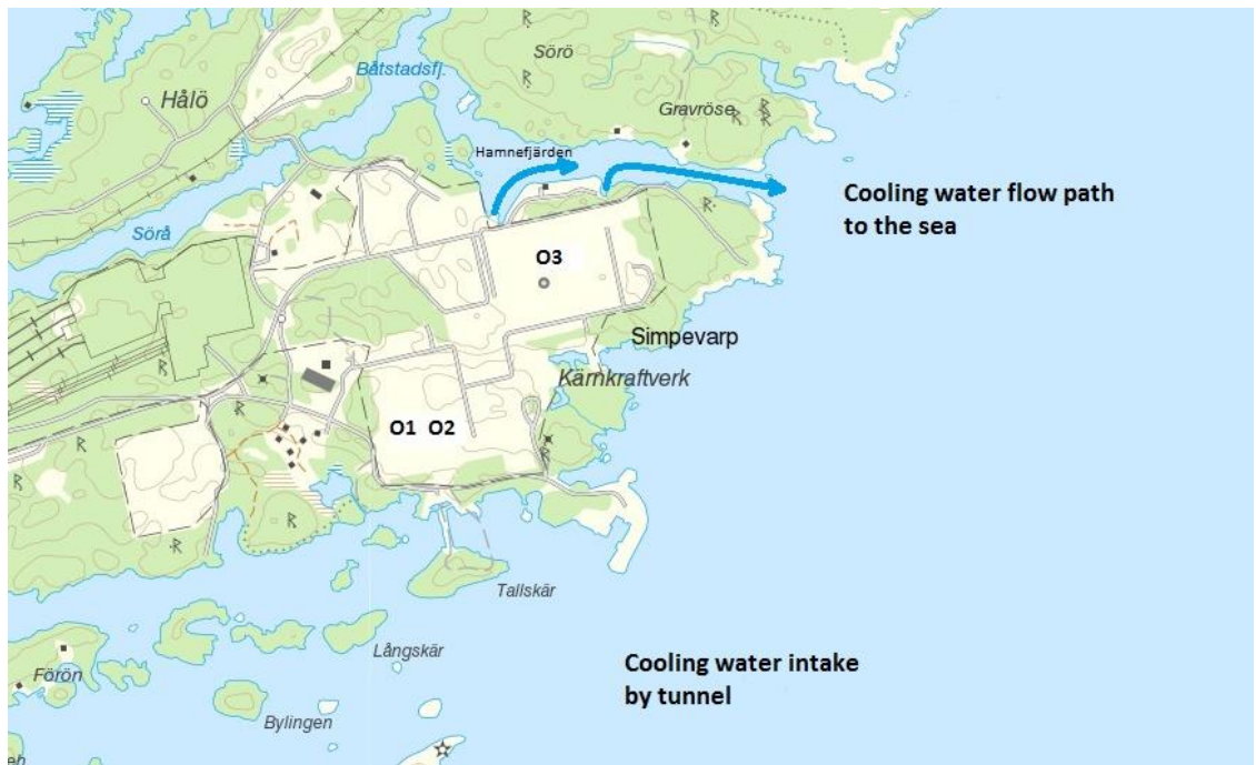
Figure 1-6. Cooling water outlet to Hamnefjärden, the left blue arrow is for Oskarshamn 1 and 2 and the right one is for Oskarshamn 3 (Lantmäteriet maps).
