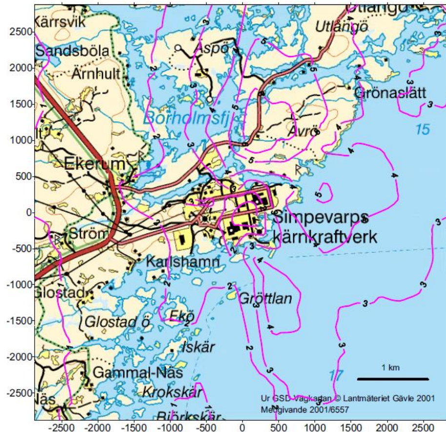
Figure 3-6. Calculated annual average concentration in air ( \text{fBq}/\text{m}^3 ) from discharge of 1 Bq, released at 70 m, i.e. from Oskarshamn 1 [30].
