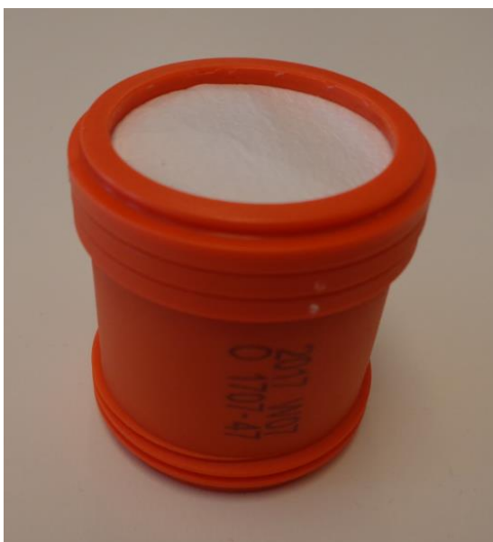
Figure 3-5. Aerosol filter used for activity monitoring in the main stacks in Oskarshamn 1 and 2.
