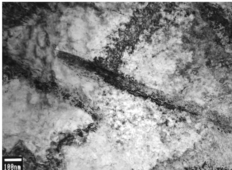
Figure 5. The microstructure in \text{Zr}_{2.5}\text{Nb} . A hydride can be seen in the middle of the figure. x80k.
