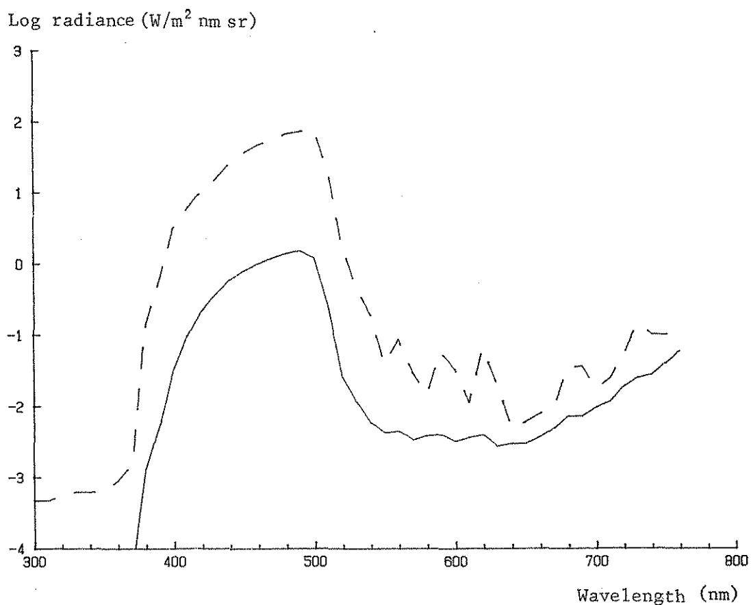
Evaluated according to A.C.G.I.H. the longest safe exposure durations are 18000 seconds (at 5 cm) to avoid burn hazards and 22000 seconds for blue light hazards. The conclusion is that the reflexes are harmless. Reflexes from curved metal surfaces of tools commonly used by dentists show figures of the same order of magnitude. Reflexes from plane, good mirrors should, however, be regarded as equal to the radiant tip itself.
