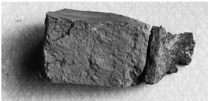
Figure 2.2.1\_2. Photograph of altered Fo-Ca 7 clay from the Stripa tests. The darkened region to the right of the sample was nearest the canister.
