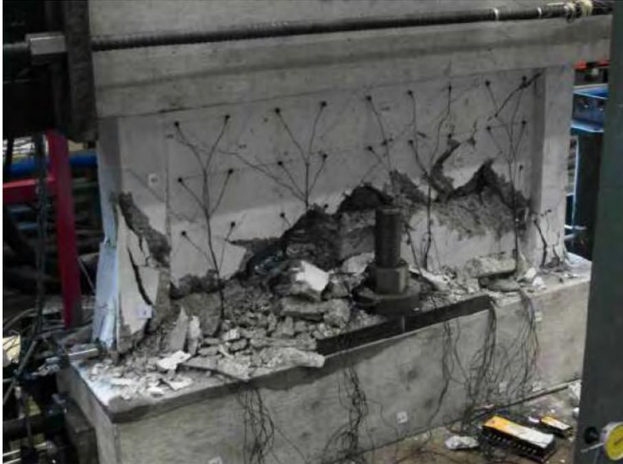
**Figure 2-11 Picture of wall specimen REG A (control specimen with normal concrete) at failure [7].**
