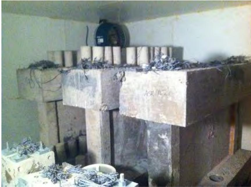
**Figure 2-3 ASR test specimens in the acceleration chamber with increased temperature and humidity [16].**
