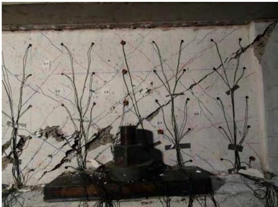
Figure 2-13 Picture of wall specimen ASR A1 (specimen with ASR reactive concrete) at failure [7].
