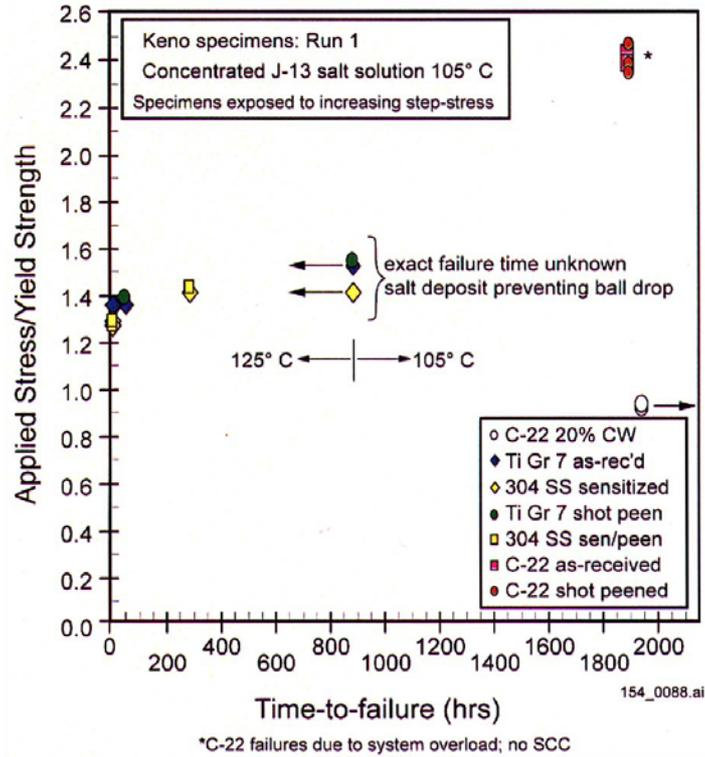
Figure 4: Constant Load (Uniaxial Tension) Stress Corrosion Crack Initiation Test No. 1
