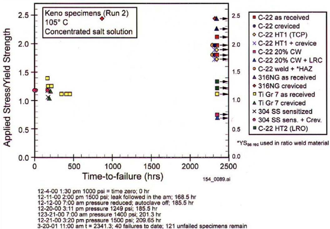
Figure 5: Constant Load (Uniaxial Tension) Stress Corrosion Crack Initiation Test No. 2
