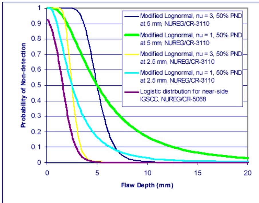
Figure 8. Probability of Non-Detection for Ultrasonic Examination from Various Sources (DOE 2000)
