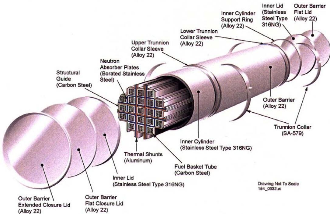
Figure 2: Typical Waste Package Designed for 21-PR Fuel Assemblies (DOE 2001a)
