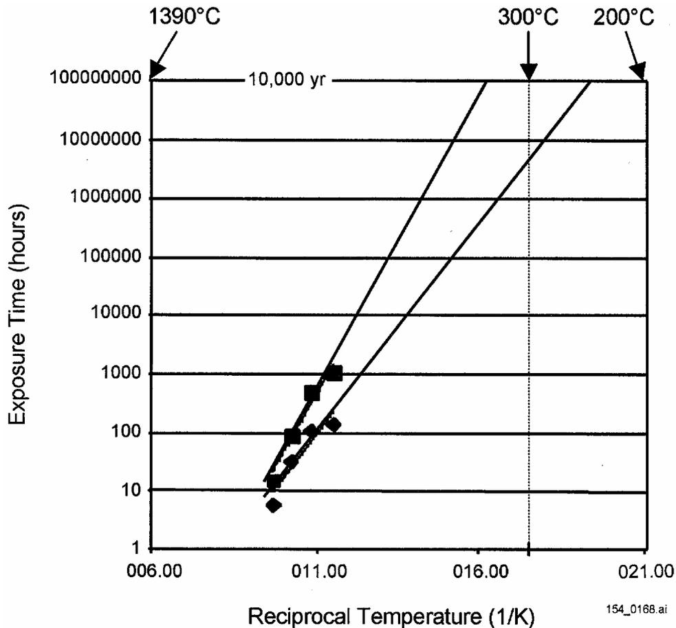
Figure 3: Extrapolation of Volume Fraction Data from Half-inch Thick, Alloy 22, Double-V, Gas-Tungsten-Arc Welds (DOE 2000)
