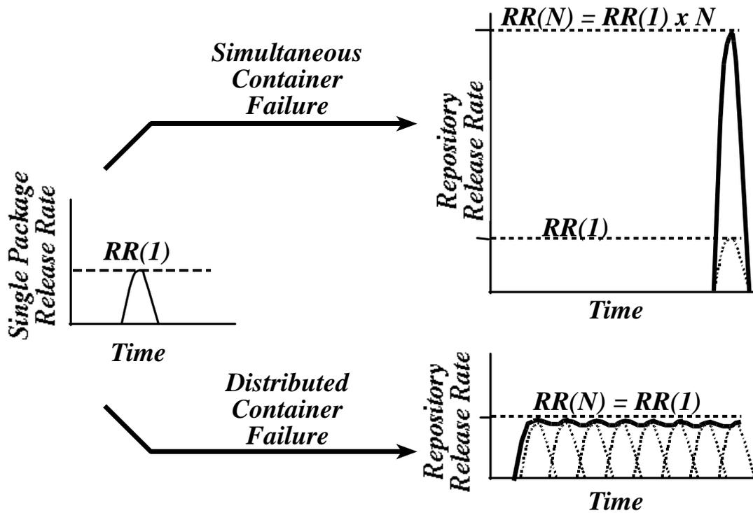
Figure A-2. Schematic Diagram of Effect of Distributed Canister Failures on Peak Release of an Instant Release Fraction (IRF) Radionuclide. "RR(1)" is a characteristic release rate curve for an IRF radionuclide from the EBS to the far-field rock (for example, Figure A-1).
