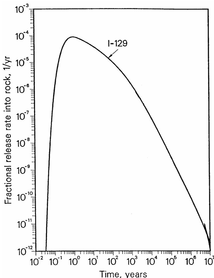
Figure A-1. Calculated Fractional Release Rate of Some Instant Release Fraction (IRF) Radionuclides Through 30-cm Thick Buffer (from Pigford et al. 1990).
