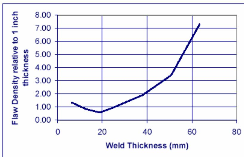
Figure 7. Effect of Weld Thickness on Flaw Density Normalized to a Thickness of 25.4 mm (DOE 2000)
