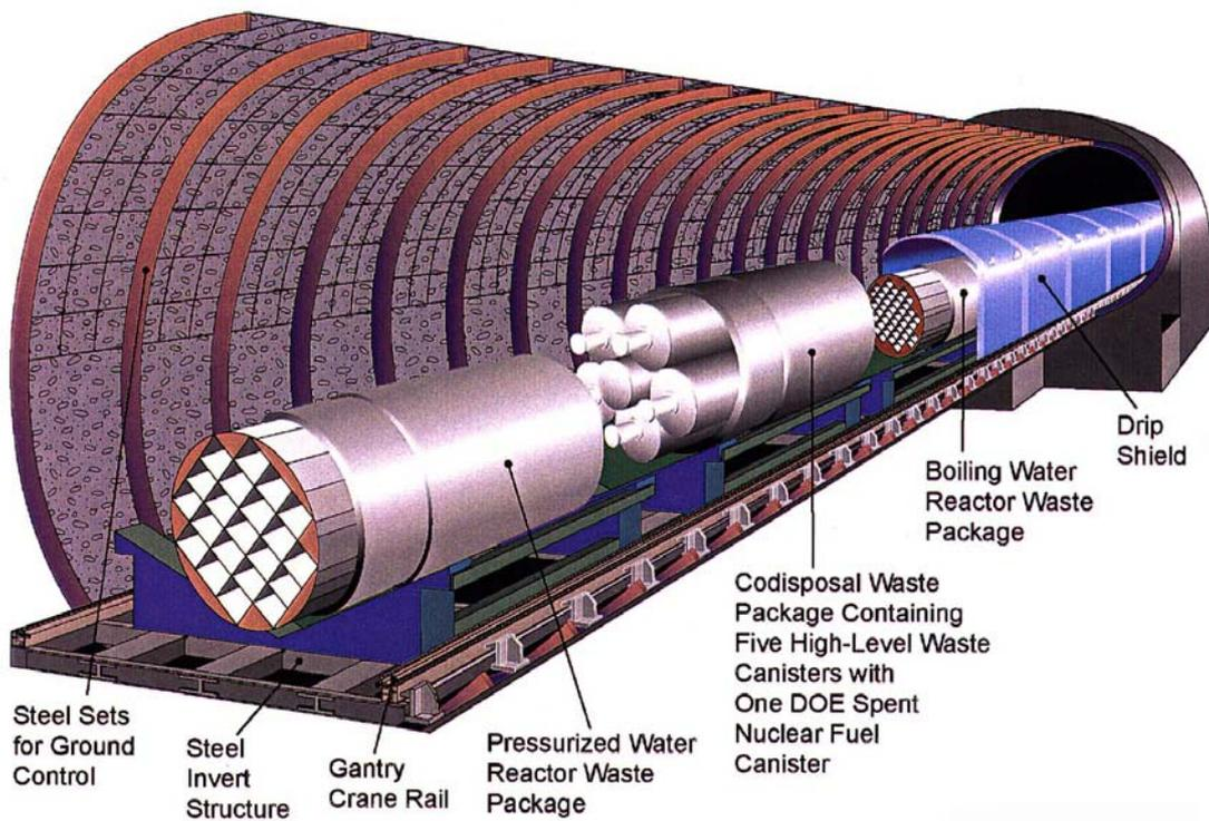
Figure 1: Arrangements for Different Types of Waste Packages and the Drip Shield in an Emplacement Drift (DOE 2001a)
