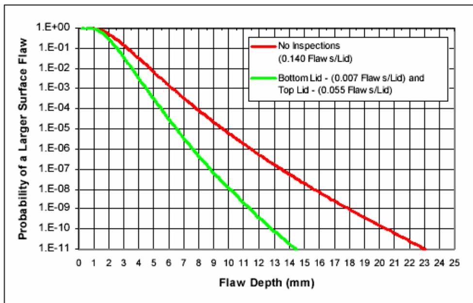
Figure 10. Size Distribution for Indicated Frequency of Occurrence of Outer Surface Breaking Flaws in Waste Package Alloy 22 Lid Welds (Monteleone 1998).
