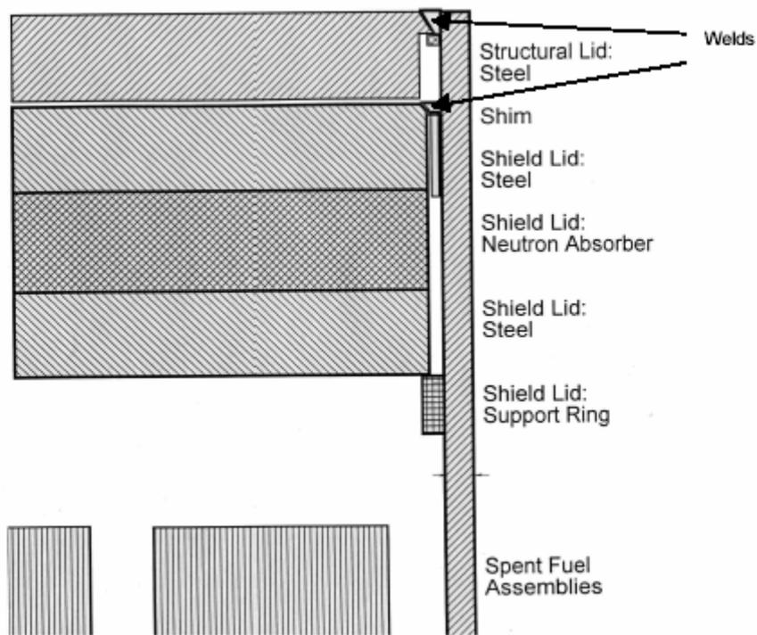
Figure 6. Illustration of Closure Welds for the VSC-24 Dry Storage Cask (DOE 2000)
