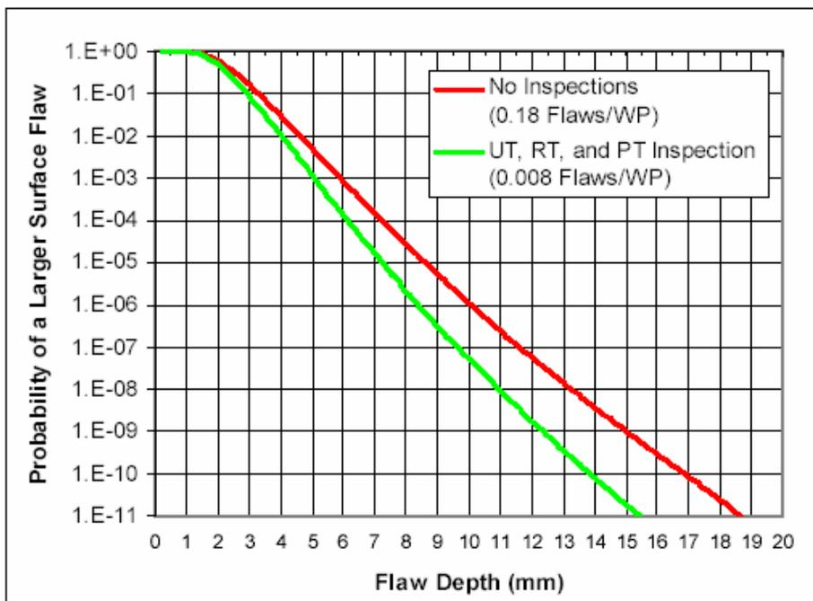
Figure 9. Size Distribution for Indicated Frequency of Occurrence for Outer Surface Breaking Flaws in Waste Package Alloy 22 Shell Welds (Monteleone 1998).
