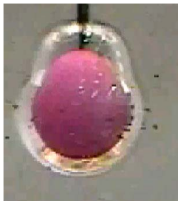
Figure 3.1: Vapor film boiling over a 10mm sphere at the subcooling of 80 K
