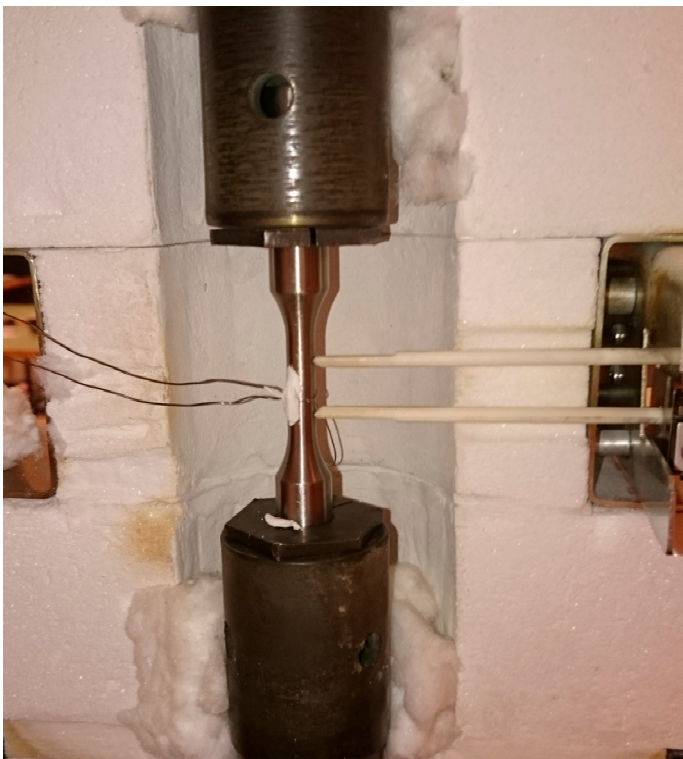
Figure 4. Test setup in oven. Thermoelements to the left, displacement gauges to the right.
